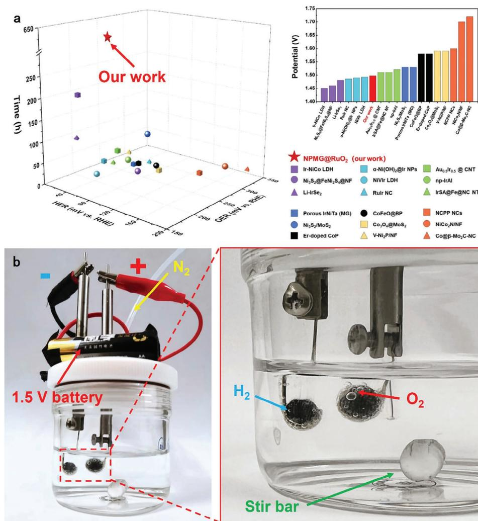
**Figure 6.** Performance comparison. a) The  $\eta_{10}$ , water splitting voltage, and long-term stability of NPMG@RuO<sub>2</sub> in HER and OER reactions were compared with those reported in the literature for electrocatalysts. More details can be found in Table S1 (Supporting Information). b) The demonstration diagram of 1.5 V battery-driven water splitting.
