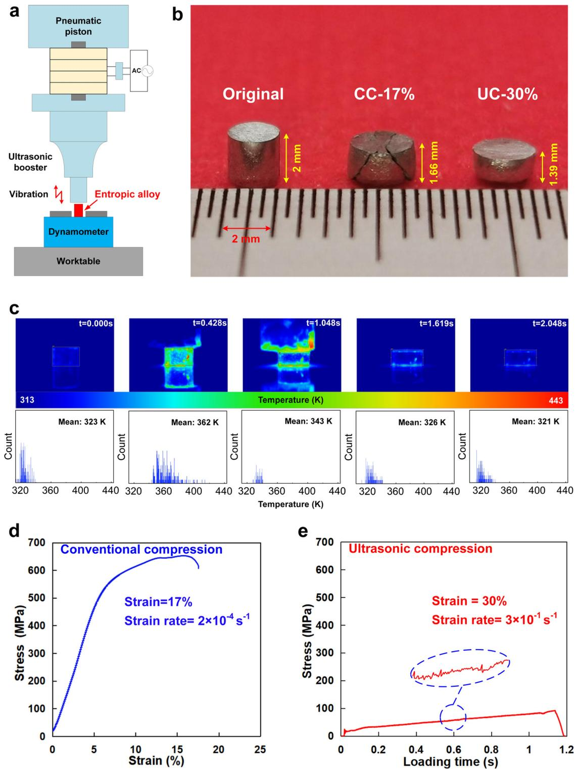
**Fig. 1.** Deformation behavior under different loading conditions. **a** Schematic of ultrasonic-assisted loading, **b** Sample deformation of conventional compression (CC) and ultrasonic compression (UC), **c** Thermal infrared images of the deformation area during ultrasonic loading, **d** Stress-strain curve of CC at room temperature, **e** Mechanical response of the entropic alloy under UC.
