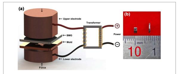
Figure 1. (a) Schematic diagram of the experimental set-up for the RWF of BMGs. (b) The photograph of the as-cast BMG (left) and the one after RWF (right).
