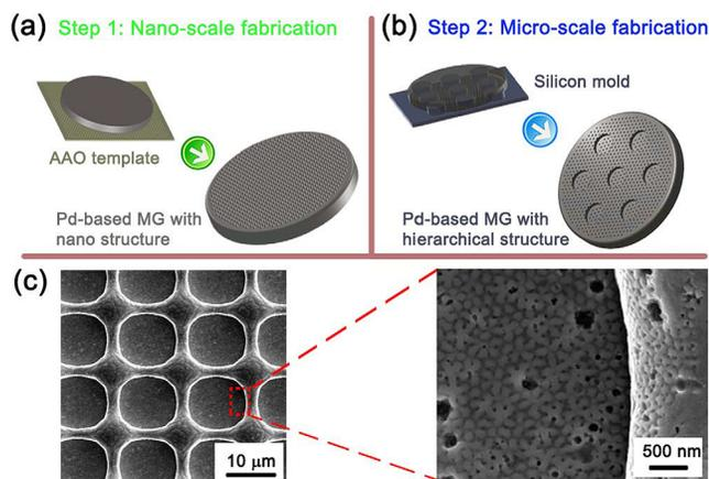
FIG. 1. Schematic diagram of the fabrication of micro-nano scale structured superhydrophobic metallic glass surface. (a) Step one: nano scale fabrication with AAO template; (b) step two: micro scale fabrication with silicon mold; (c) SEM images of the as-fabricated MG surface (left) and the magnified details (right).
