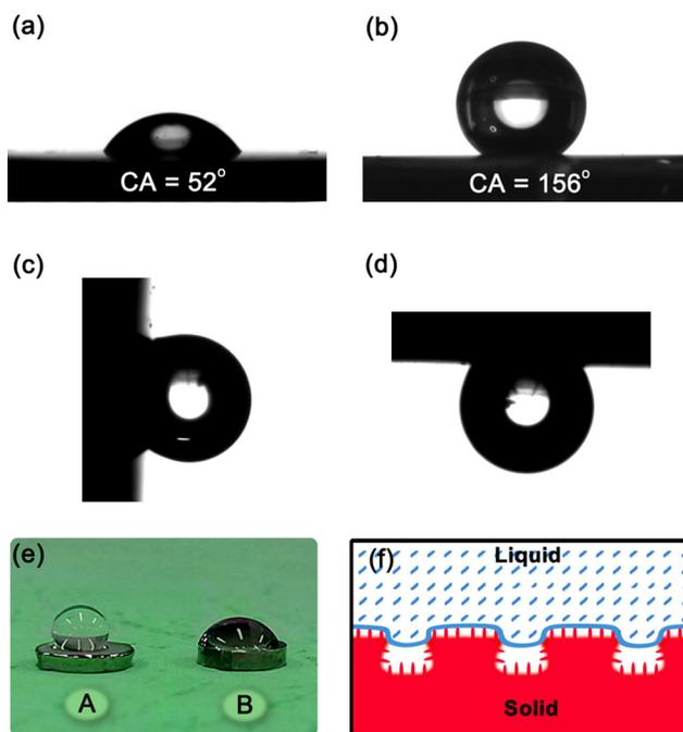
FIG. 2. (a) and (b) The CAs of the polished and micro-nano hierarchical surfaces of Pd-based MG, respectively. (c) and (d) The shapes of water droplet on the MG surface with tilted angles of  $90^\circ$  and  $180^\circ$ . (e) The photographs of water droplets on the two different surfaces, A: the micro-nano hierarchical surface and B: the polished one. (f) The wetting regime.
