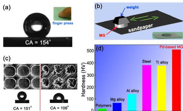
FIG. 3. Mechanical stability of the hierarchical MG surface. (a) The CA of micro-nano hierarchical Pd-based MG surface after finger press. (b) Illustration of the scratch test on sandpaper (2000 mesh). (c) The SEM images and CAs before and after the damage of the hierarchical structure by sandpaper abrasion test. (d) Hardness comparison of Pd-based MG, polymers and some crystal alloys.
