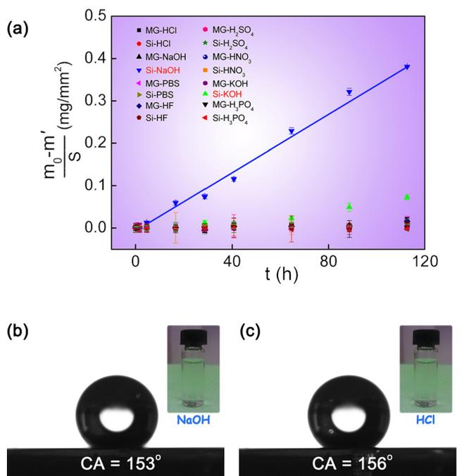
FIG. 4. (a) Mass loss of silicon and MG on per unit area in different corrosion solutions with the increase of time. (b) and (c) The CAs of micro-nano hierarchical Pd-based MG surface after soaked in the NaOH solution (1 mol/l) and the HCl solution (1 mol/l) for about 120 h.
